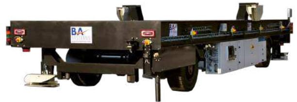
The HLT can handle 18 pallets simultaneously. Flexible, the shuttle can be equipped with a refrigerated box equipped with motorized chain or roller conveyors or with a simple platform for manual or automatic loading. Provided with AGV Manager, a fleet management software, designed and developed by BA Systèmes, an HLT10 type of AGV fleet interfaces directly with the customer's plant management tool.
