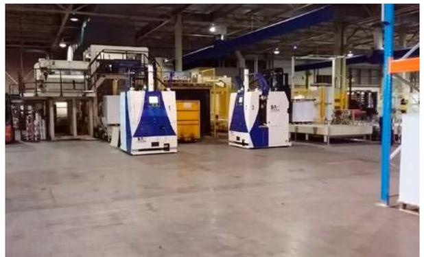
The turnkey solution developed by BA Systèmes was based on a thorough logistic analysis, conducted in close cooperation with Sappi. BA Systèmes has integrated the system into the heart of Sappi's production process, comprising of 7 AGVs, an automatic battery changing system (Autoswap), and the AGVs' traffic management through AGV Manager, BA Systèmes' supervision system. The contract also included the supply of pallet racking systems and the connection to existing and new conveyor systems.
